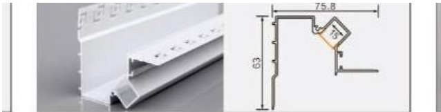
XT831 7564 indirect light L × 75.8 × 63 mm 15 mm flexible LED strip
