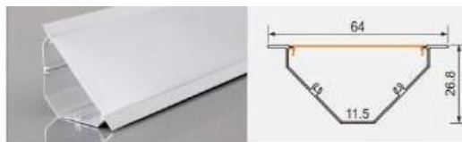
XT-913 6427 crown molding L × 64 × 26.8 mm 11 mm flexible LED strip
