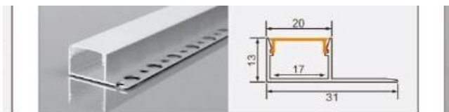
XT764 Single-row perforated 20, single-bottom trim L × 31 × 13 mm 17 mm flexible LED strip / rigid LED bar
