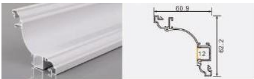
XT823 6261 crown molding L × 60.9 × 62.2 mm 21 mm flexible LED strip
