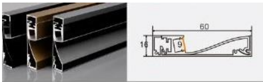
XT635+636 6016 skirting L × 60 × 16 mm 9 mm flexible LED strip
