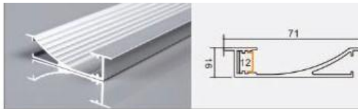
XT328 7116 skirting L × 71 × 16 mm 12 mm flexible LED strip
