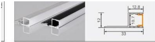
XT703 13 side trim L × 33 × 12 mm 10 mm flexible LED strip
