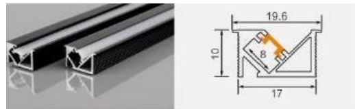
JP20 1710 with flange, angled light L × 19.6 × 10 mm 8 mm flexible LED strip
