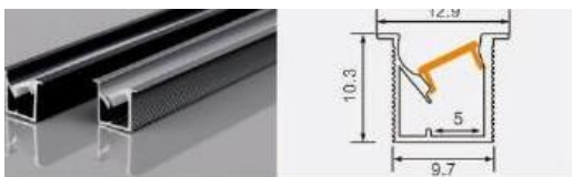
JP08 1010 with flange, angled light L × 12.9 × 10.3 mm 5 mm flexible LED strip
