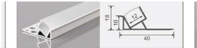
XT-870 4018 L × 40 × 18 mm 12 mm flexible LED strip
