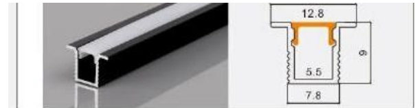
XT293 0809 with flange L × 12.8 × 9 mm 5.5 mm flexible LED strip / rigid LED bar
