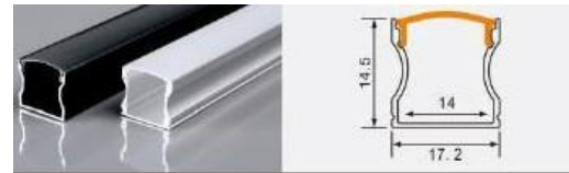
XT393 1715 L × 17.2 × 14.5 mm 12 mm flexible LED strip / rigid LED bar
