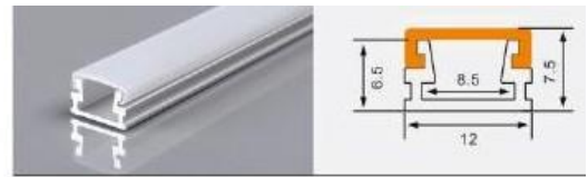
XT268 1208 L × 12 × 7.5 mm 8.5 mm flexible LED strip / rigid LED bar
