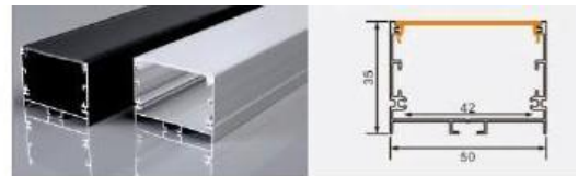
BG85 5035 L × 50 × 35 mm 42 mm flexible LED strip / rigid LED bar
