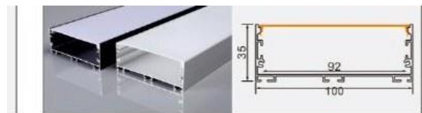
BG56 10035 L × 100 × 35 mm 92 mm flexible LED strip / rigid LED bar
