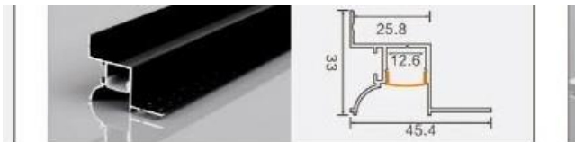
XT825 4533 indirect light, plaster L × 45.4 × 33 mm 12 mm flexible LED strip
