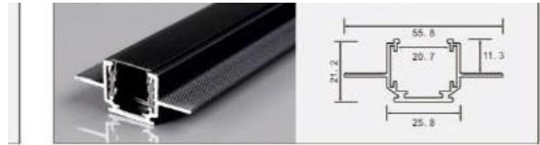
WR-CX-45 Recessed L × 55.8 × 21.1 mm 1.6 magnetic-attraction light
