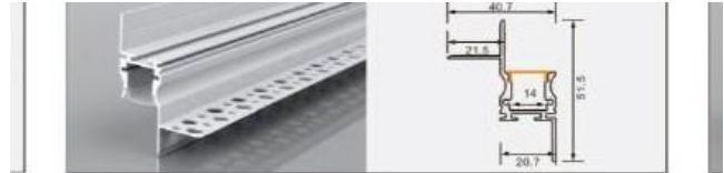
XT800 4152 panel clamp L × 40.7 × 51.5 mm 14 mm flexible LED strip
