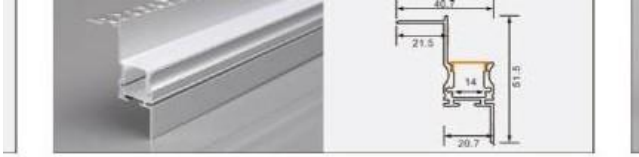
XT630 4152 plaster L × 40.7 × 51.5 mm 14 mm flexible LED strip
