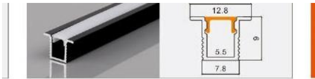
XT293 0809 with flange L × 12.8 × 9 mm 5 mm flexible LED strip
