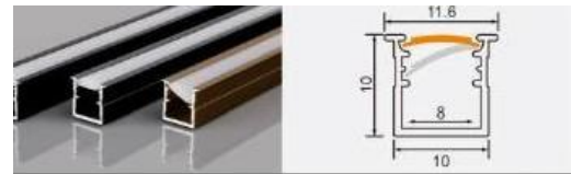
JP29 Weld-free 1010 with flange L × 11.6 × 10 mm 8 mm flexible LED strip / rigid LED bar
