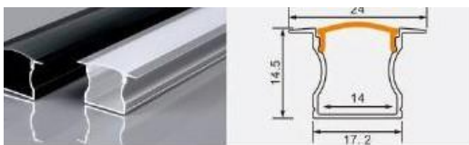
XT394 1715 with flange L × 24 × 14.5 mm 12 mm flexible LED strip / rigid LED bar
