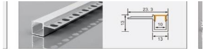
XT756 Single-row perforated 13, single-top trim L × 23.3 × 13 mm 10 mm flexible LED strip / rigid LED bar
